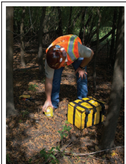
Seismic nodes' small footprint makes them ideal for ecologically sensitive areas and urban environments.
