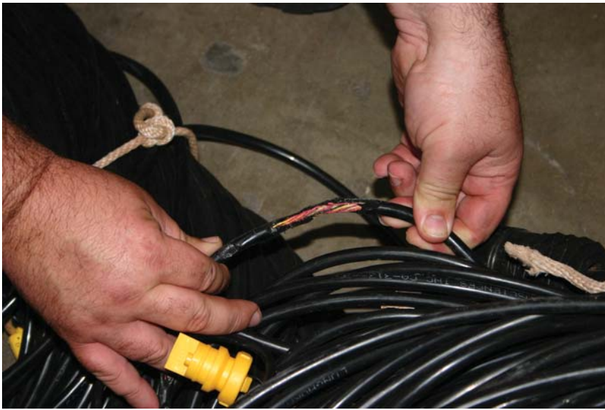
Cable-free acquisition systems eliminate potential damage or other problems to cables and connectors—the most vulnerable link in a conventional seismic surveying system. The technology also dramatically reduces weight and logistical requirements while offering unlimited expansion and improved surveying productivity.
