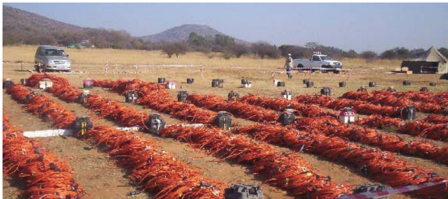
Figure 2. This image shows the typical spread cables used by today's cable telemetry systems to communicate from the various remote units to the central recorder via an interconnecting cable. Although the occasional optical or RF repeater may be used to overcome obstructions, the system communicates entirely via cables. The cables may use twisted-pair copper or fiber optics as the telemetry medium.
