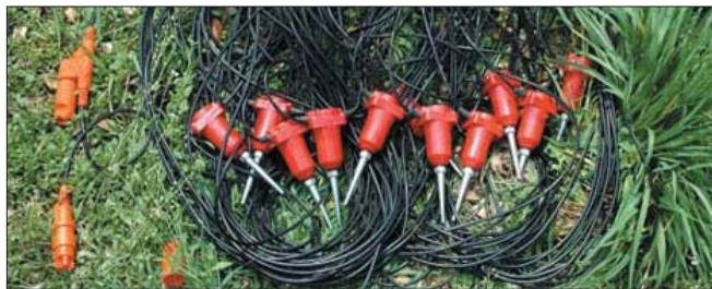
Figure 1. Geophone string with connectors.
